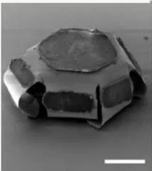
When an open theragripper, left, is exposed to internal body temperatures, it closes on the intestinal wall. In the gripper's center is a space for a small dose of a drug.
